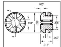
**EAR Equipment Feet:** Replaces standard single screw mount rubber feet commonly found on most audio equipment. Formed from black EAR Isodamp C1002 material. MF-1010 are 1.0" D x .5" H, accept 3mm D screw, load range 5-15 pounds... 75¢ each - L-021 are 1.5" D x .75" H, accept 5mm D screw, load range 10-20 pounds... \$3.50 each
