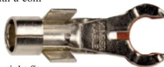
Available either in unplated copper or with Kimber's proprietary *Ultraplate* finish, **PM-25** fits 1/4" posts, **PM-33** fits 5/16" posts, overall width is .535", accepts up to six gauge wire. Supplied with heat shrink & Wonder solder. Specify unplated copper or *Ultraplate* finish and size....
