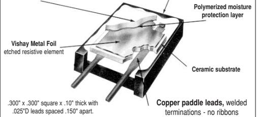
Vishay 1280G trimming potentiometers: Bulk metal foil pc mount type, much superior to any cermet or conductive plastic trimmer, the best available... .75W, 15ppm, 26 turns for ultra-precise adjustment... \$12.50 each except  $10\Omega$  @\$13.50
